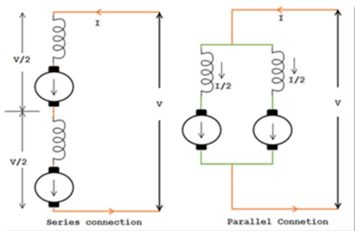
To control the DC series motor this is another way called series parallel technique. This is the method normally used in traction by connecting two or more than that of the series motor are couple mechanically at the same load.
