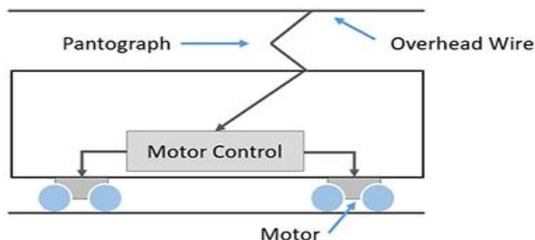
This type of DC supply is supplied to the vehicle through two different ways:
